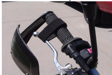
Front Brake Strap Lock
